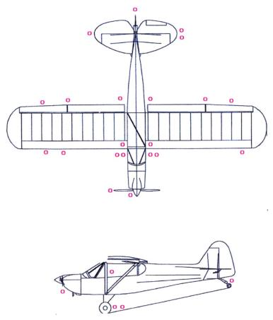
**Note**: Visually check the airplane for general condition during the walk around inspection. In cold weather remove even small accumulations of frost, ice, or snow on the wing, tail, and control surfaces. Also, make sure that the control rods and cables are free of ice and move freely.
